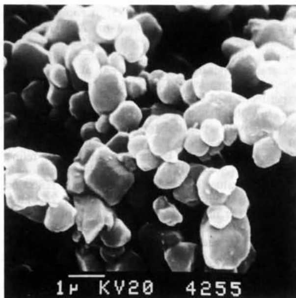
Fig. 1. Scanning electron micrograph of the pollucite analogue \text{Cs}_2\text{CuSi}_5\text{O}_{12} .
